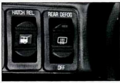
To turn on the rear window defogger, find the switch marked REAR DEFOG on your instrument panel to the left of the steering column. Press the top of this switch until the light in the switch comes on, then release it.
